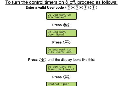
Use keys 1 - 8 to toggle control timers on and off
